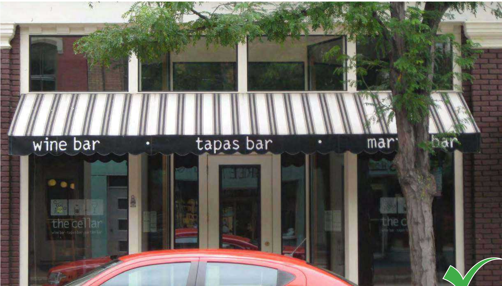
Lettering on the valance (fringe) of the awning should contrast with the fabric color for legibility.
